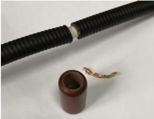
Picture 2: using corrugated coaxial cable to build a loop antenna
