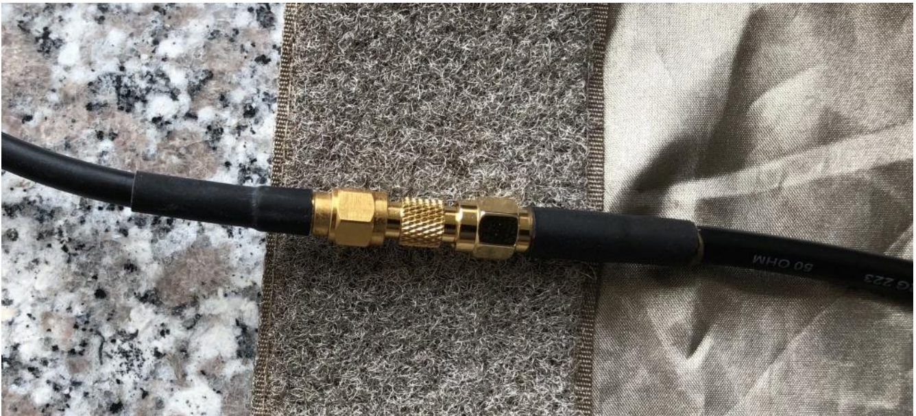
Picture 9: feed through using coaxial adapter
