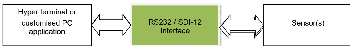
Figure 2 – TBS06-TS basic application setup
