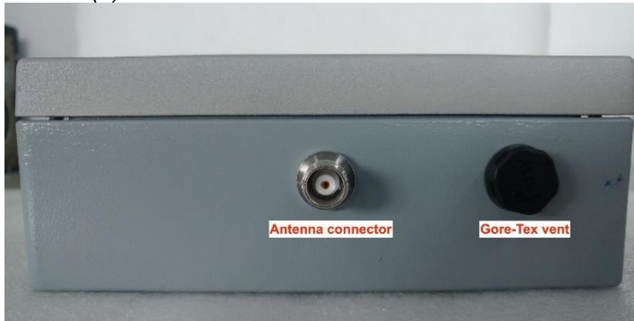
(3) TBSL1: antenna connector and vent
