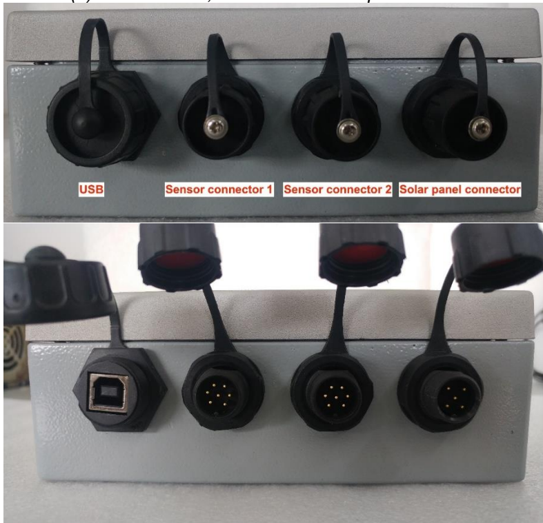
(2) TBSL1: USB, sensors and solar panel connectors
