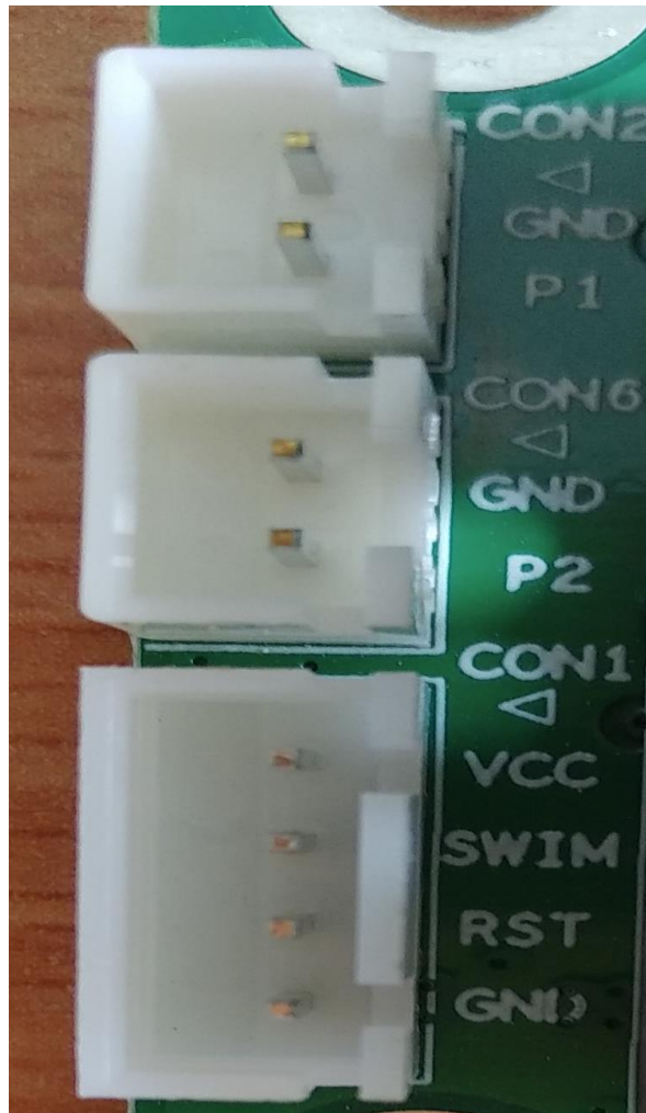
Pulse inputs and SWIM connector – pins description
