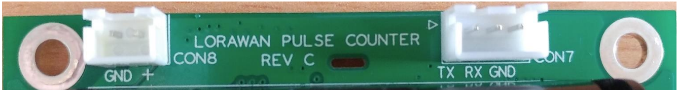
External power supply and debug UART connectors – pins description
