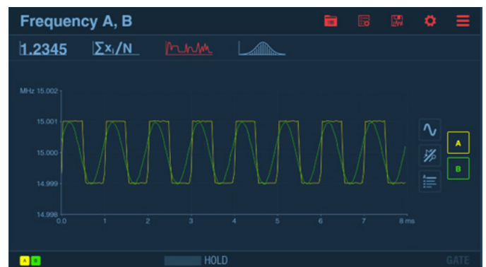
View fast FM, or any time/phase/frequency modulation, on screen, on one or two channels. Here we see FM modulation with both sine and square wave shape
