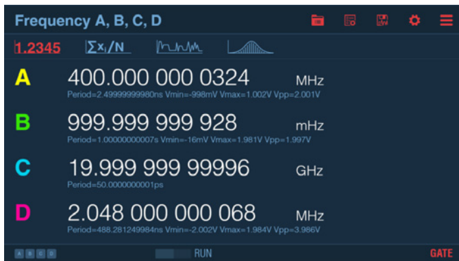
VALUES display mode: Compare 4 signals simultaneously on screen, with auxiliary parameters below. No need for a DVM, or oscilloscope, to check amplitude!
