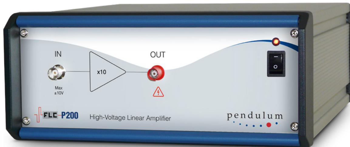
The Pendulum Instruments High Voltage High Current Linear Amplifier P200 has a fixed amplification of 10 times and capable of bipolar high voltage output of  $\pm 100$  V. Any signal source with amplitude up to  $\pm 10$  V can be used as an input device. The input amplitude should normally be kept within  $\pm 10$  V. The High Voltage High Current Linear Amplifier P200 is equipped with a microfuse rated at 40 mA, which will be blown if the input voltage exceeds 300% of the maximum.
