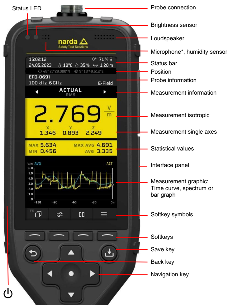
Fig. 2. FieldMan display and controls
