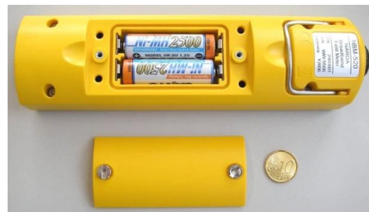
The battery compartment is opened easily using a coin. Two replaceable NiMH rechargeable batteries (AA size) are used to power the device.
