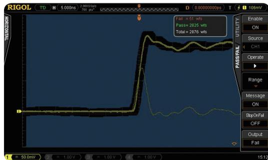
User-defined mask, Pass/Fail counts, stop on fail, fail alarm
