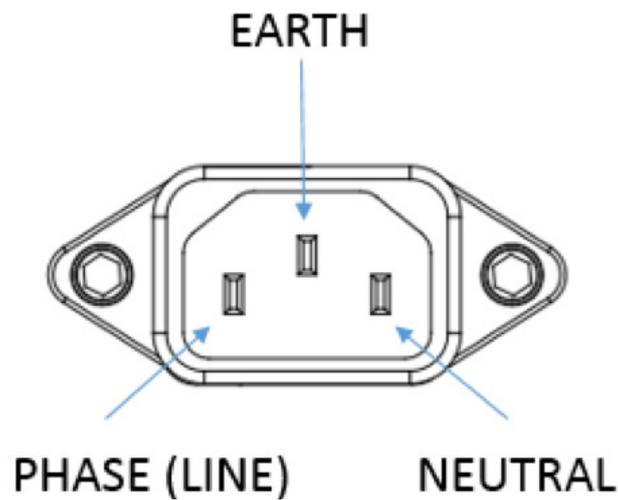
Figure 7 – Mains connector, pin assignment \*)
