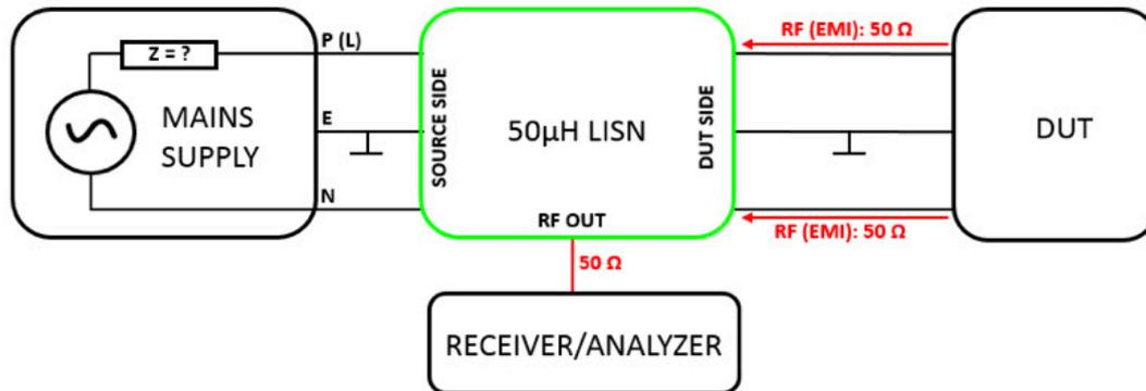
Figure 1 – Basic AC LISN set up: impedance levels.
