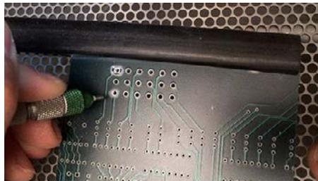
The Coating Removal System CRS9000 is a self-contained workstation designed for the safe removal of conformal coatings from printed circuit boards and other electronic devices.
