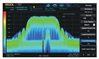
With the Density spectrum, you can find out the exceptional signals hidden behind the high-level signals, and capture them accurately with the FMT.
