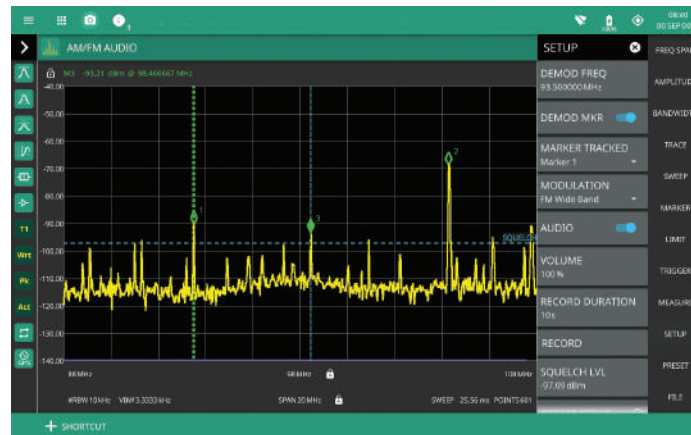
AM/FM Signal Demodulation at Marker Frequency
