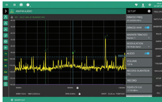
AM/FM Signal Demodulation at Marker Frequency
