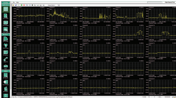
View the Spectrum Traces from Multiple MS27200As on a Single PC Monitor with the Vision High-Speed Port Scanner Option
